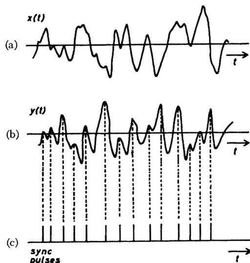
Fig. 3. Maximal-value triggering. (a)  $x$ -signal, to be processed. (b)  $y$ -signal. (c) Series of sync pulses.
