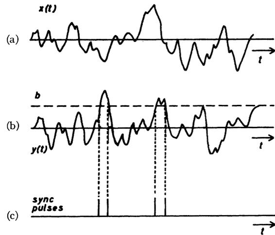
Fig. 1. Dual-polarity triggering. (a)  $x$ -signal, to be processed. (b)  $y$ -signal and threshold level  $b$ . (c) Series of sync pulses.
