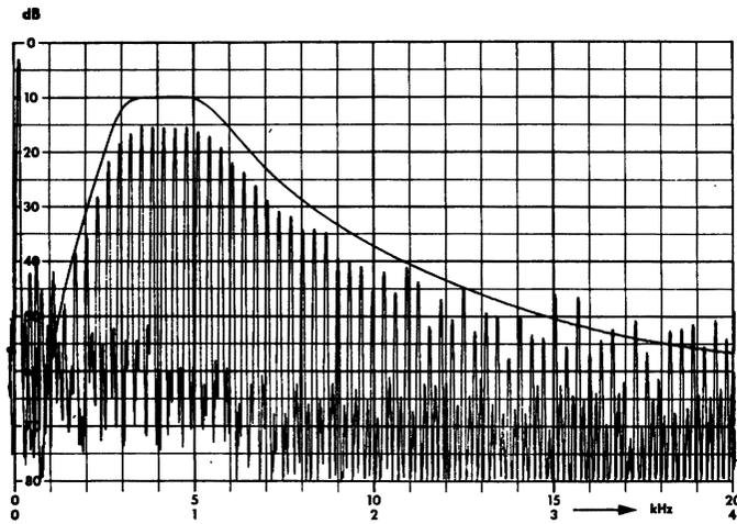
Fig. 5. Spectrum associated with the result shown in Fig. 4, above. The measured correlation function was scanned 64 times/second. Full-drawn line: frequency response of the filter as measured directly (with proper driving and load resistances) by combination of Rohde and Schwarz Audio-Frequency Spectrograph type FNA and the associated Synchronous Oscillator. Full width of spectrum: 4 kHz, linearly divided. Vertical scale in decibels.
