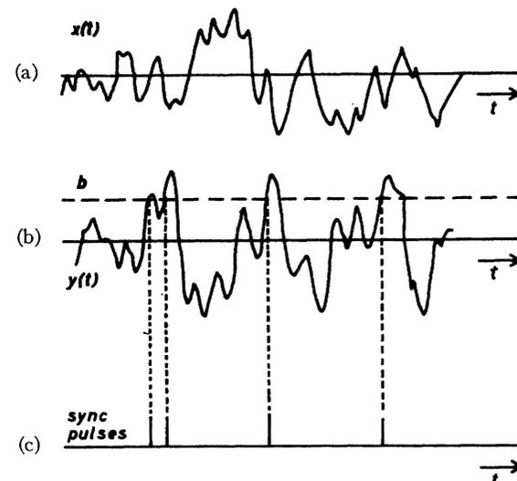
Fig. 2. Single-polarity triggering. (a)  $x$ -signal, to be processed. (b)  $y$ -signal and threshold level  $b$ . (c) Series of sync pulses.
